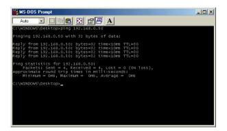
Access Point. A good wireless connection will show four replies from the wireless router or access point, as shown.
