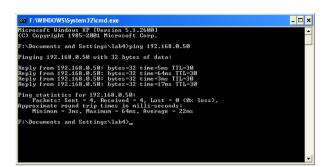
Access Point. A good wireless connection will show four replies from the Wireless Router or Access Point, as shown.
